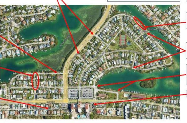
In design for a stormwater improvement project for the Lido and 45<sup>th</sup> Ave neighborhood. Feasibility study showed a gravity system would not work and a pump station alternative is being designed.
